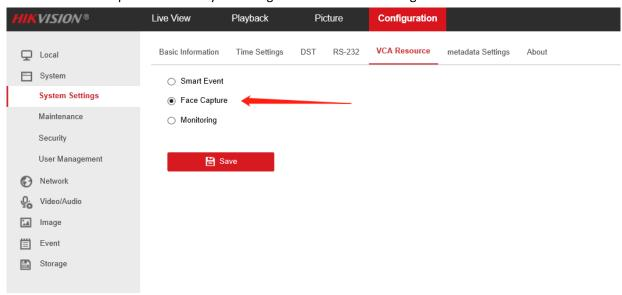
b. Face Capture mode include sending the mask wearing attributes, BUT **DON'T** support the mask detection alarm by the camera itself. The attributes can be sent to the NVR or the HCP and the alarm can be realized by them.
