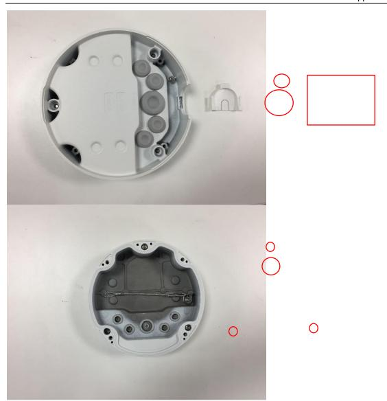
**Step3:** fixed camera: Hook up the bullet camera's cramp ring use antistripping cable from junction box to prevent the camera from falling off during installation, after connecting the reticle and power line, use four screws to fix the camera to the junction box.
