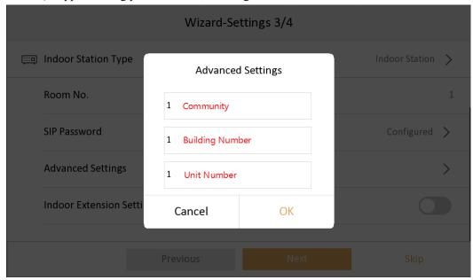
2) Support remote configuration of indoor extension information through the main indoor station;
