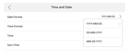
2) Support the Settings->General Settings->Time and Date interface, set the 12-hour system, 24-hour system two formats, and the default setting is 24-hour system display.
