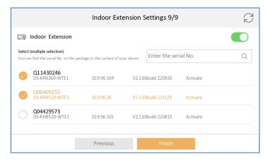
D. Pairing with main door station, sub door station and indoor extension *Note*: The pairing time duration depends on the device quantity you selected in previous steps, it will take about up to 5 mins, please wait patiently until the process finish and show "Configured" as below.
