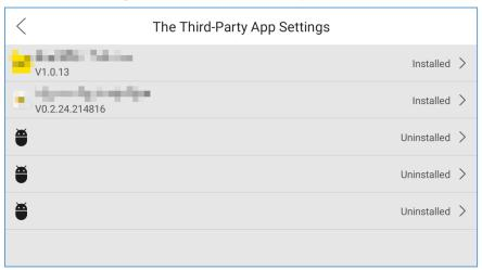
3. Support installing 3<sup>rd</sup> APP via TF card, copy apk file to TF card, and select from indoor station and install.
