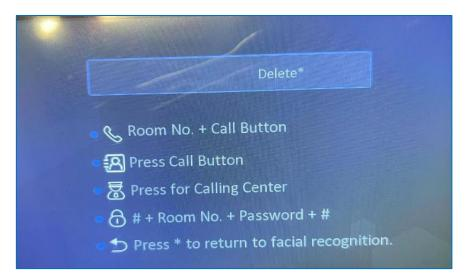
10. Press \* and # simultaneously, after input the password and the device will enter the admin configuration page.
