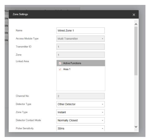
It supports detector type, Zone type, Detector Contact Mode and Pulse Sensitivity. Wired zone support Dual zone.
