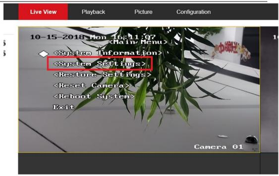
2. You can switch options by adjusting UP and DOWN of PTZ, and click Iris+ to confirm.
