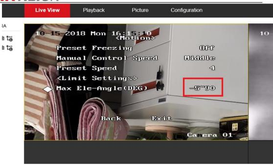
6. Choose the Max Ele-Angle(DEG) and click Iris+ to confirm, the diamond on the left will get hollow, then you can click UP and DOWN to adjust it from -5~90° to -90~90° (actually the effect
