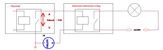
Connection two: connection method for external extension relay
