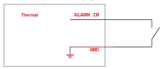
Alarm input connection method
