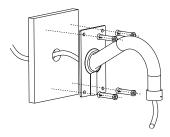
4 Finish wiring, install the dome core on the change over bowl and adjust camera angle.
