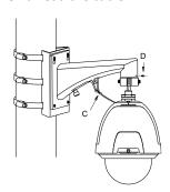
C: Safety rope D: Tightening screw
