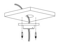
3 Thread the wire and fix the speed dome to bracket
