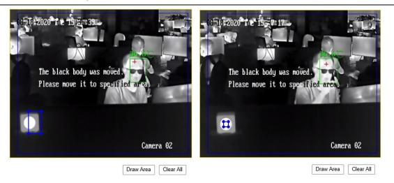
**Note:** This alarm only showed by thermal channel OSD information, could not be transferred to back-end devices or platforms as a type of event.
