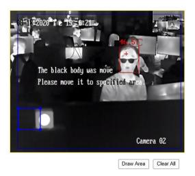
In addition, the black body should be included in the blue frame completely. If not, this OSD alarm would also be triggered.
