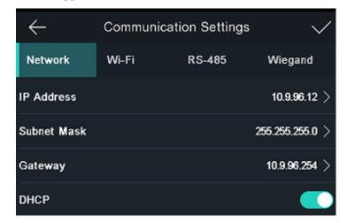
Note: face terminal and thermal module communicate internally with IP address 192.168.1.2 and 192.168.1.64, don't use these two IP address for device and PC in case of IP conflict. Don't set IP address 192.168.1.64 for terminal, or thermal module will become offline. and don't set IP address 192.168.1.2 for PC/server, or device cannot communicate with PC/server.
